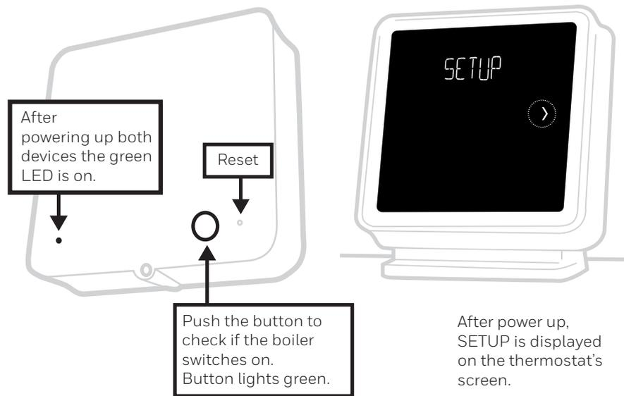
After power up, SETUP is displayed on the thermostat's screen.
