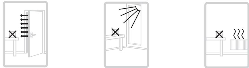
The T6R thermostat should not be placed near draughts, in direct sunlight or near heat sources.
