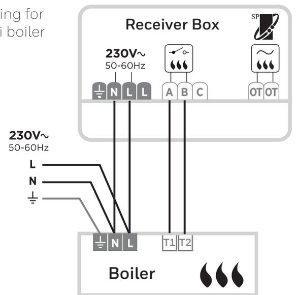
**C)** Wiring for OpenTherm boiler
