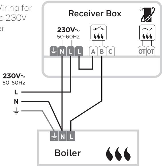
**B)** Wiring for Combi boiler
