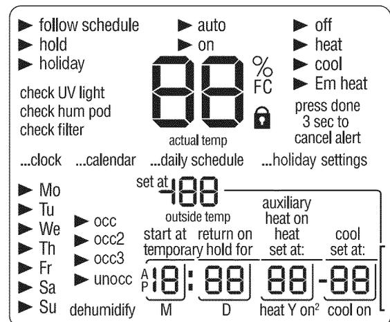
Fig. 1 — Thermostat Display
