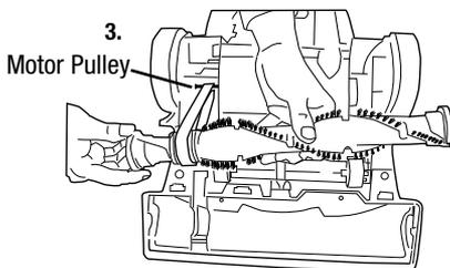
4. Pull the rotating floor brush firmly into position, stretching the drive belt, and place ends of rotating floor brush down into the slots on sides as shown. Alignment of brush ends in slots may be necessary to fully insert the brush.
